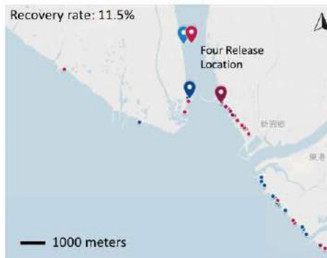
▲ Figure 5. The recovery map of wood drifters released after rainfall and on a non-rainy day. Two release locations (light blue and pink) are on the bridge that is about 2 km from the estuary; the others (dark blue and dark purple) were at a coastline about 1 km from the estuary.
