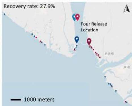
▲ Figure 5. The recovery map of wood drifters released after rainfall and on a non-rainy day. Two release locations (light blue and pink) are on the bridge that is about 2 km from the estuary; the others (dark blue and dark purple) were at a coastline about 1 km from the estuary.
